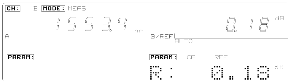
Figure 2-5. Measuring the Reflection Reference
